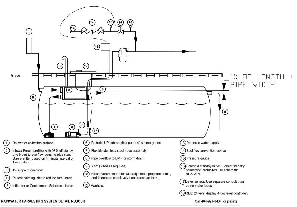
BELOW-GROUND TANK WITH SUBMERSIBLE PUMP, PRESSURE TANK, NO FILTRATION, SOLENOID STANDBY WATER SUPPLY NOT TO SCALE
