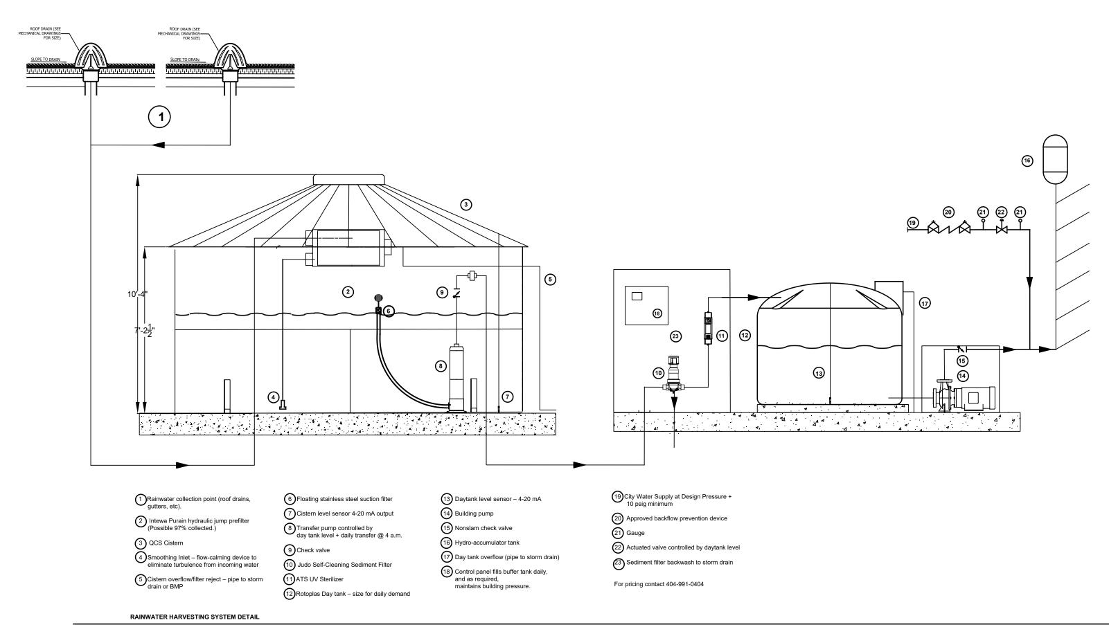
ABOVE GROUND TANK, END SUCTION TRANSFER PUMP, UV TREATMENT, DAY TANK, END SUCTION BUILDING PUMP WITH HYDRO-ACCUMULATOR, PRV STANDBY CONNECTION
