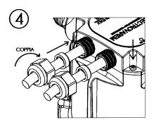
Clamp the cable glands with a maximum permissible torque: **3.5 Nm**
