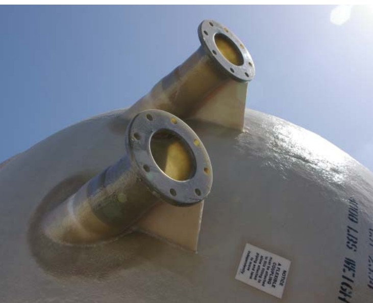
▼ FIBERGLASS NOZZLES AND PVC PIPING
